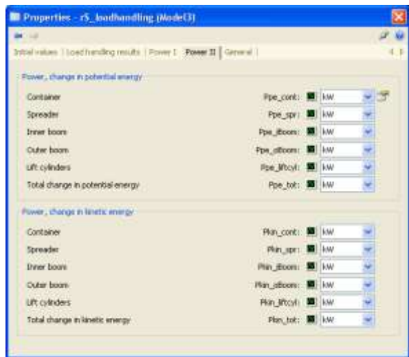
Figure 23. The power II results tab of the reach stacker MBS element type.
