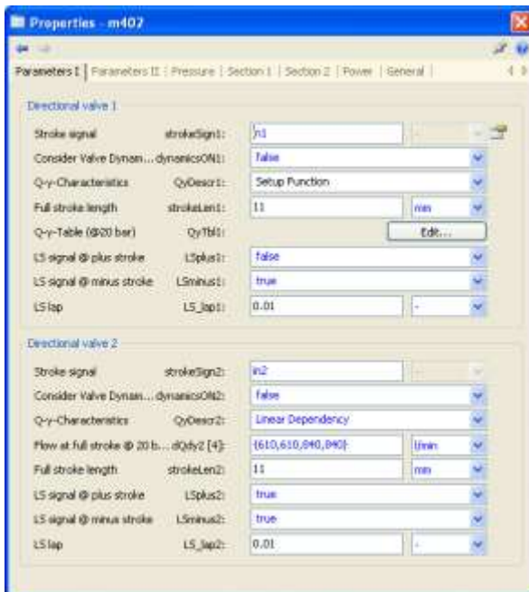
Figure 14. The parameters I tab of the M402 directional control valve element type.
