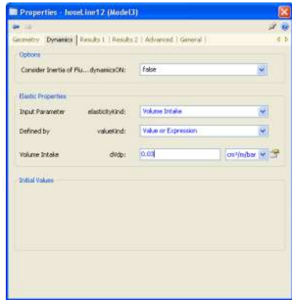
Figure 27. The dynamics tab of the hose element type.
