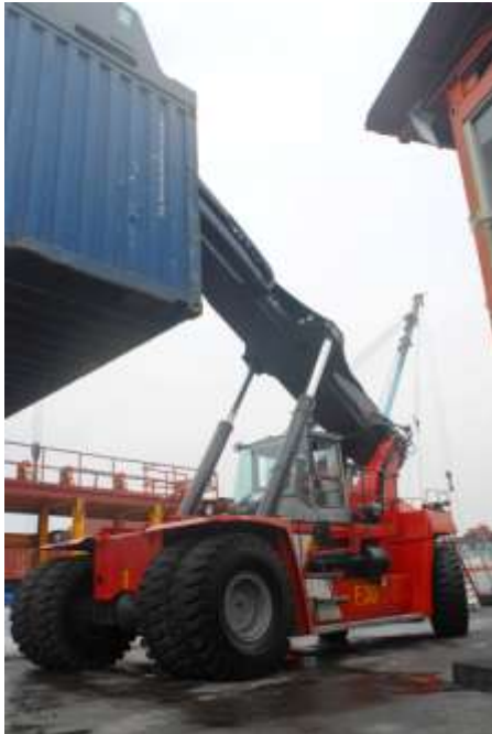
Figure 1. Kalmar DRF450 reach stacker [2].
