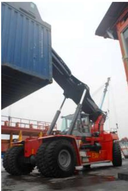
Figure 1. Kalmar DRF450 reach stacker [4].
